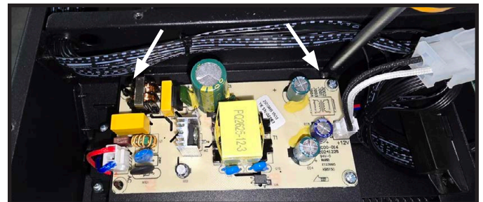
Figure 18 Cream Control Board Removal
