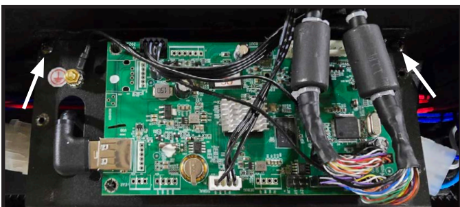
Figure 17 Computer Board Assembly Removal
