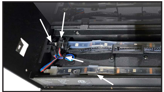
Figure 5 Ember Bed LED Wire Harnesses
