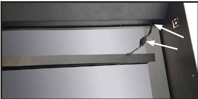
Figure 4 Downlight Wire Harness
