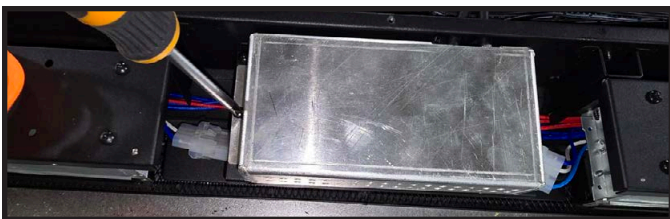
Figure 16 Computer Board Metal Shroud Removal
