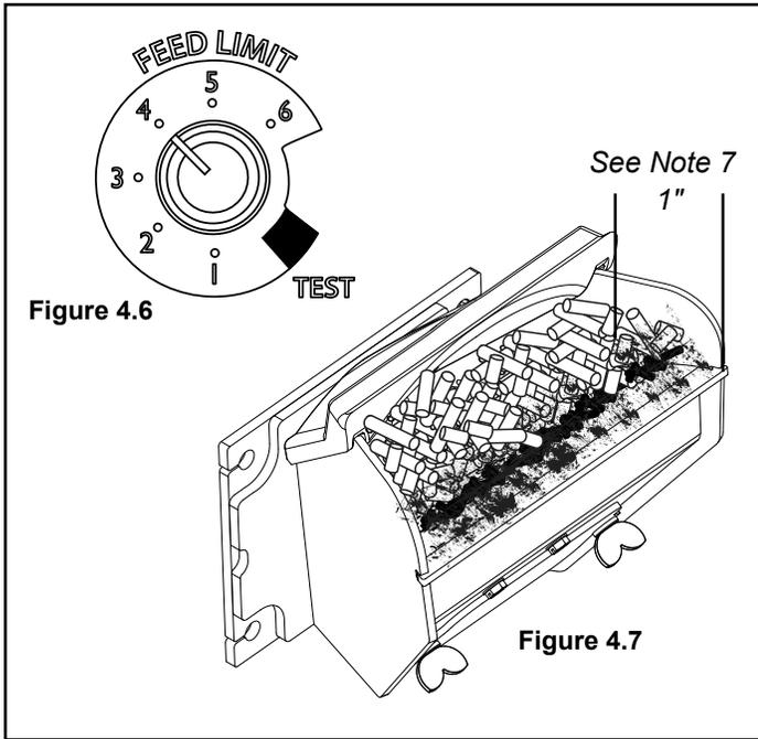
1. *Fines are small pieces of broken pellets (sawdust). Fines do not flow easily and often build up on the hopper funnel bottom angles. These fines can be pushed into the feeder opening and then fill the hopper with pellets. As the system works, they will be burned.*
