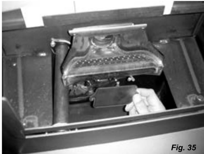
Igniter hot lead wires
