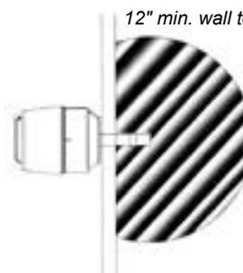
36" min clearance to any combustible material
