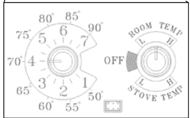
**Room Temperature Mode:** This setting, see above, will produce a room temperature of 70 degrees with the distribution blower at medium speed.
