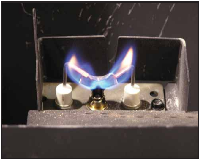
Figure 3.1 IPI Pilot Flame Patterns
