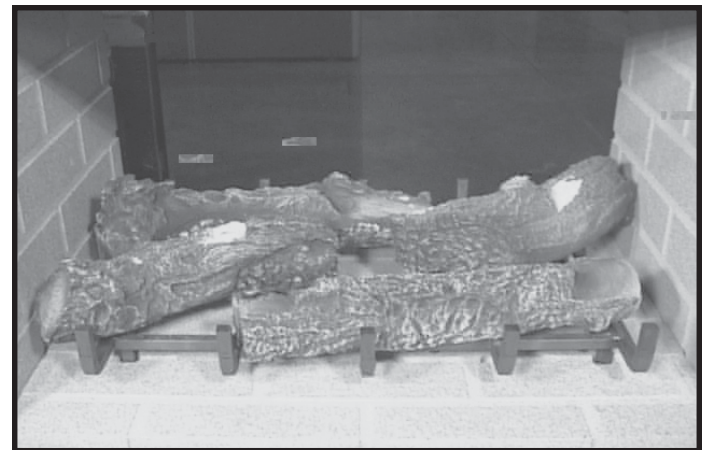
LOG NUMBER 4 (SRV675-723): Place log #4 so that the slot on the bottom of the log fits over the grate tab on the front left corner of the grate. The right end of log #4 must rest against the stop of the left center bar.
