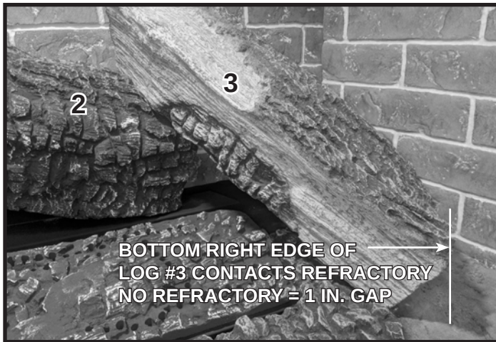
Figure 5 Place Log #3 (LOGS-6K / LOGS6KX / LOGS-6-BIR)
