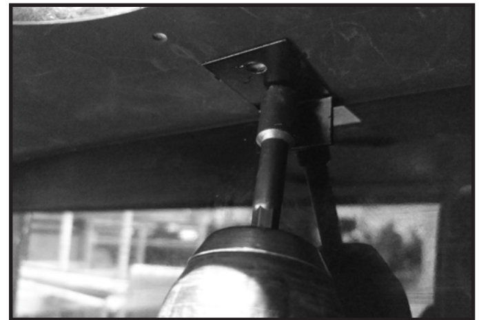
Figure 11.6 Retaining Bracket Installation - Back
