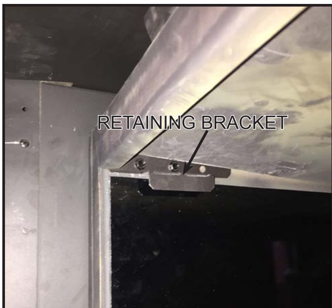
Figure 11.8 Retaining Bracket Installation - Side Panel
