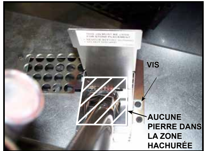
Figure 11.14 Support de placement des pierres
