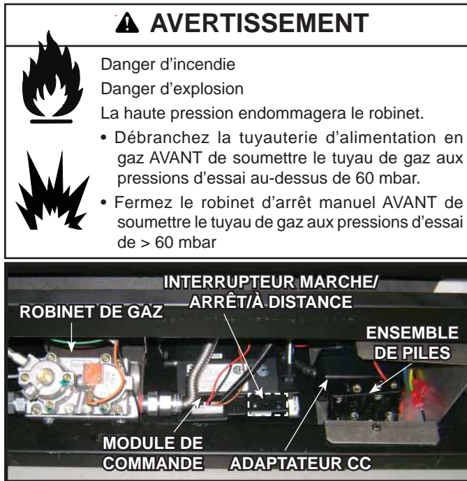
Figure 11.1 Composants du robinet
