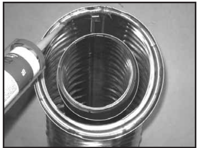
Figure 10.2 High Temperature Silicone Sealant (149 °C (300 °F) minimum continuous exposure rating)
