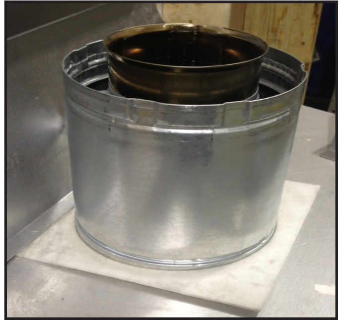
Figure 9.2 To attach the first section of vent pipe, make sure to use the fiberglass gasket to seal between the first vent component and the outer fireplace wrap. Use 2 self tapping screws to secure the gasket to the outer wrap.
