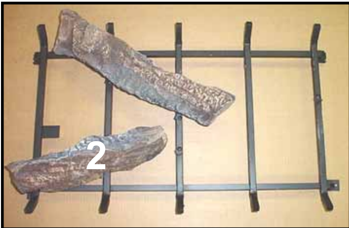
LOG #2 (SRV2068-701): Locate log #2 in left front corner of the log grate using bottom grooves for placement. Push log against grate tabs on first and second bars.
