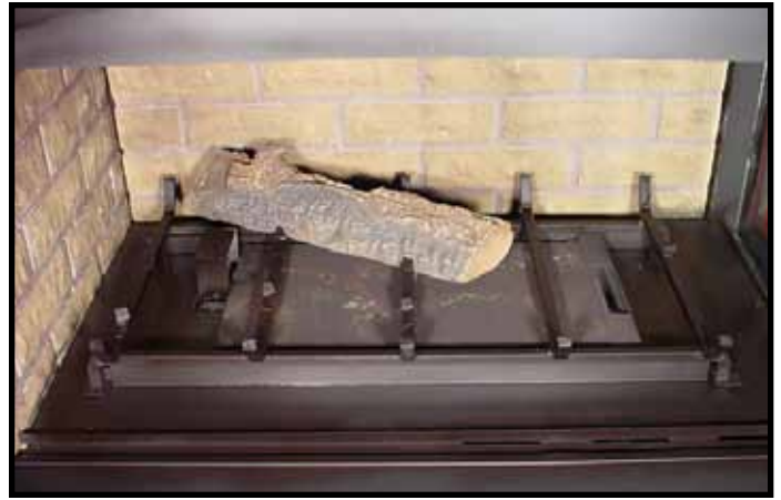
LOG #1 (SRV2068-700): Place log #1 behind grate tabs on the second and third grate bars on the left rear corner. Position so that the bottom grooves fit over bars and the log is snug against the grate tabs.
