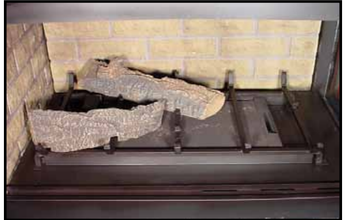
LOG #2 (SRV2068-701): Locate log #2 in left front corner of the log grate using bottom grooves for placement. Push log against grate tabs on first and second bars.
