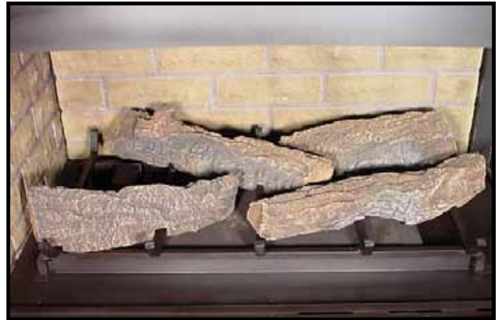
LOG #4 (SRV2068-703): Place log #4 in the right rear corner of the log grate using bottom grooves for placement. Align log #4 by using the grate corner and rear cross bar as stops.
