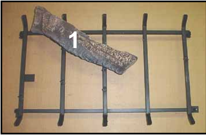
LOG #1 (SRV2068-700): Place log #1 behind grate tabs on the second and third grate bars on the left rear corner. Position so that the bottom grooves fit over bars and the log is snug against the grate tabs.
