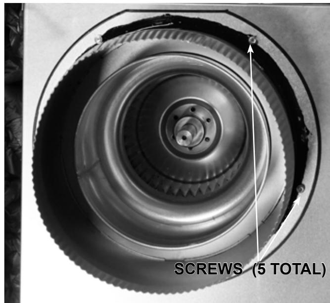
Figure 8F.4 Base Plate Fastened to Intake
