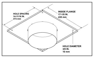
Figure 8D.2 10 Inch Chimney Collar Dimensions (RS14)
