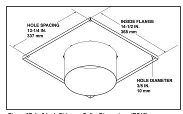
Figure 8D.1 8 Inch Chimney Collar Dimensions (RS12)
