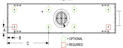
The hood shall be supported at specific locations using 1/4-20 UNC threaded rods. Qty 2 threaded rods are required in the front and back left hand corner
