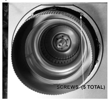
Figure 8F.4 Base Plate Fastened to Intake
