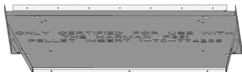
**CAUTION! Use care when installing tek screws, do not strip the holes.**
