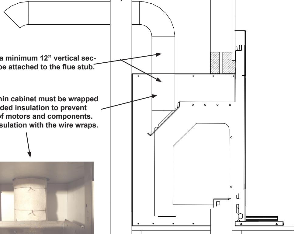
**Start the insulation with this point in the rear of the flue stub. The insulation will wrap two times around the pipe. Secure it in place with the two pieces of wire supplied.**
