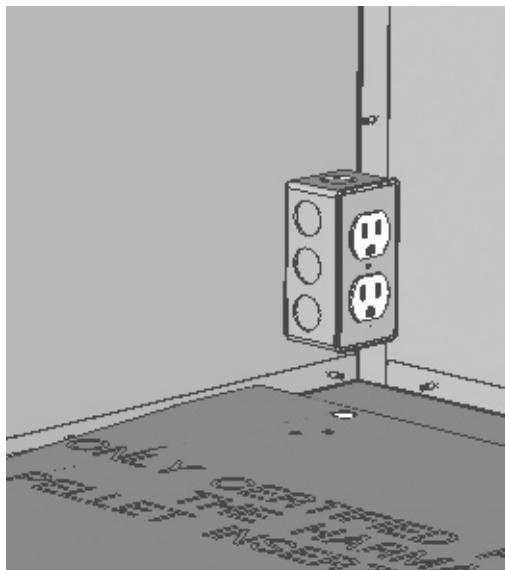
A knockout is provided in the left rear corner of the zero clearance cabinet to install an electrical outlet (not supplied) if desired. Be sure to ground the receptacle to the zero clearance cabinet if installed.
