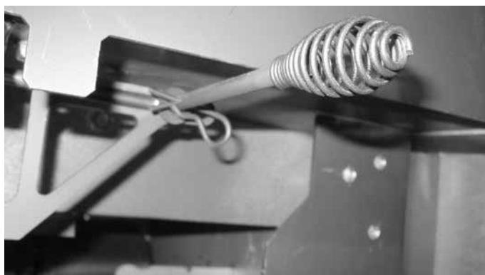
Figure 4.36 Reinstalling Hairpin Clip and Washer
