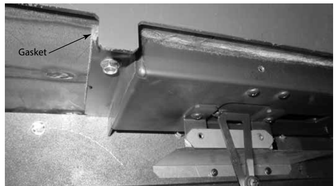
Figure 4.22 Install New Air Chamber
