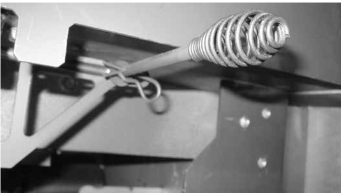
Figure 4.25 Reinstalling Hairpin Clip and Washer
