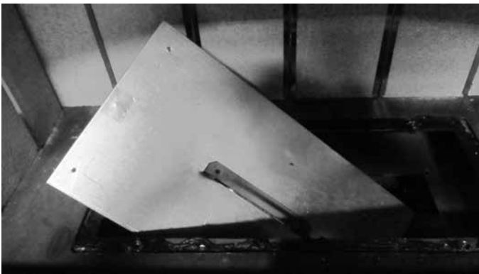
Figure 4.12 Removal of Combustion Cover
