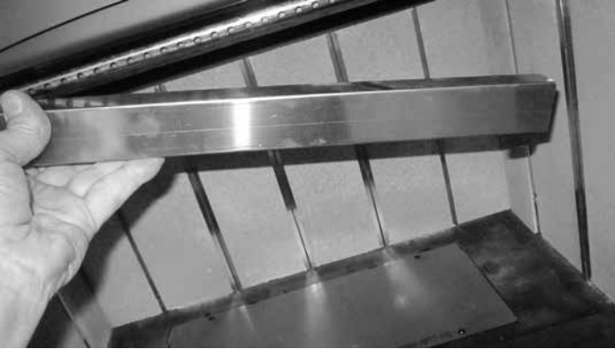
Figure 4.5 Removing Baffle Protection Channel
