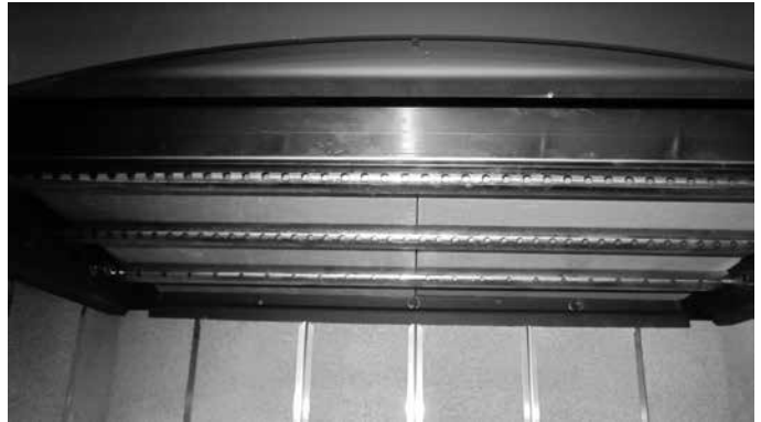
Figure 4.8 Reinstall Baffle Boards
