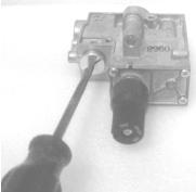
STEP 2: Screw the solenoid into the opening to attach to the valve.
