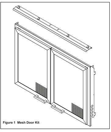
**CAUTION!** The door kit is heavy. We recommend two installers to put the front assembly in place.
