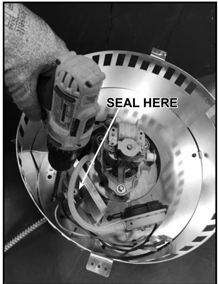
Figure 3.13 Attach Wire Harness Bracket to Bottom Dish
