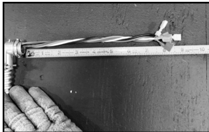
Figure 3.9 Sufficient Wire Extending Through Bracket
