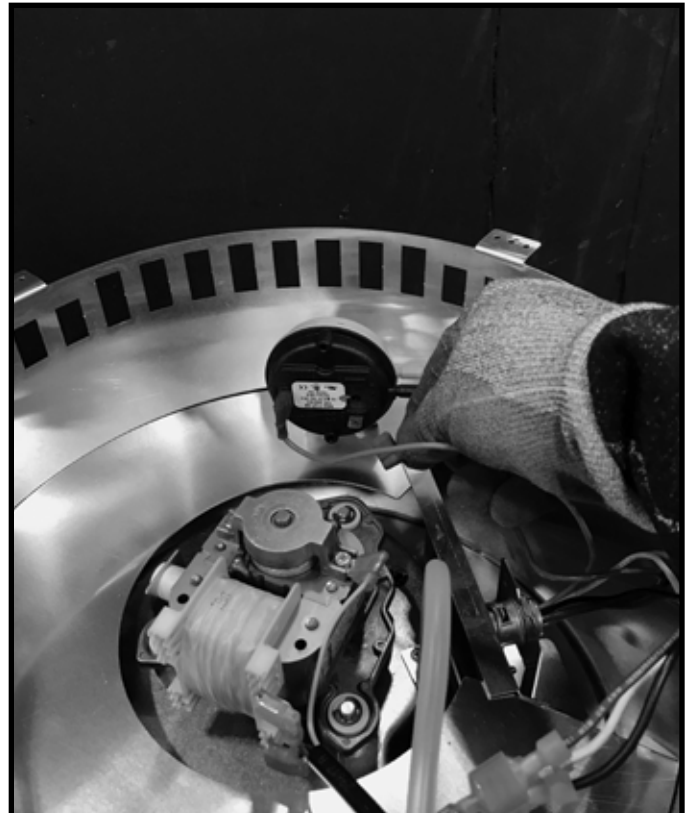
Figure 5.3 Remove Wires from Pressure Switch
