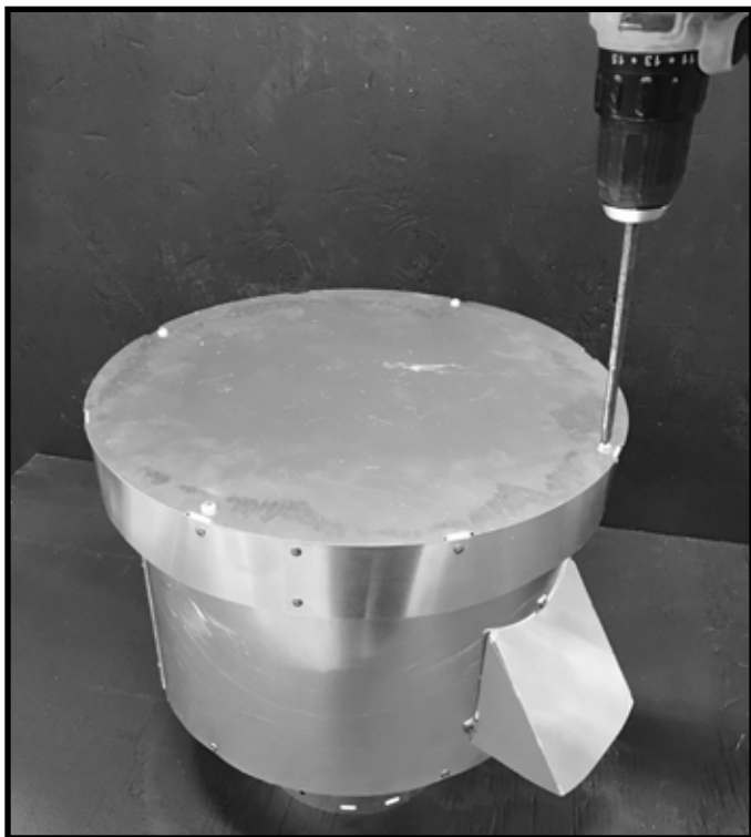
Figure 3.6 Remove Top Cap Screws
