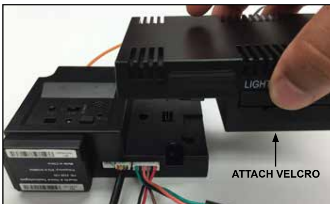
Figure 4.3 Connecting IFT-ACM and IFT-ECM
