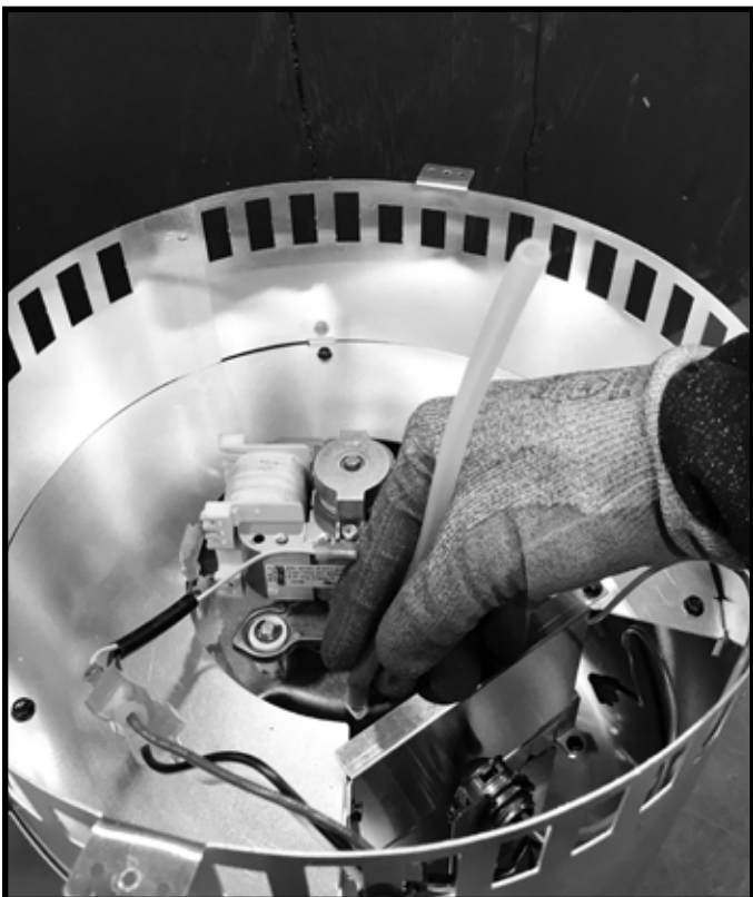
Figure 5.5 Remove Teflon Tubing from Blower
