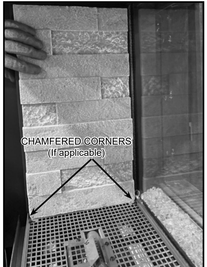
Figure 16 Positioned Side Refractory Panel
