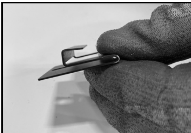
Figure 6 Refractory Bracket Prepared
