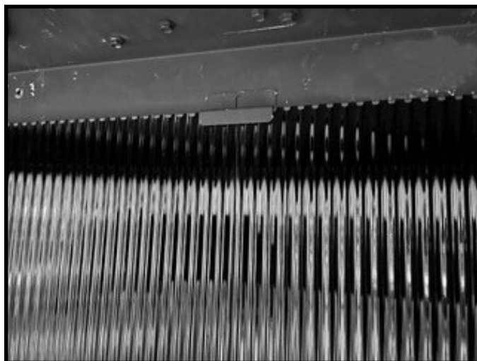
Figure 20 Install Refractory Brackets on Back Panel Seams
