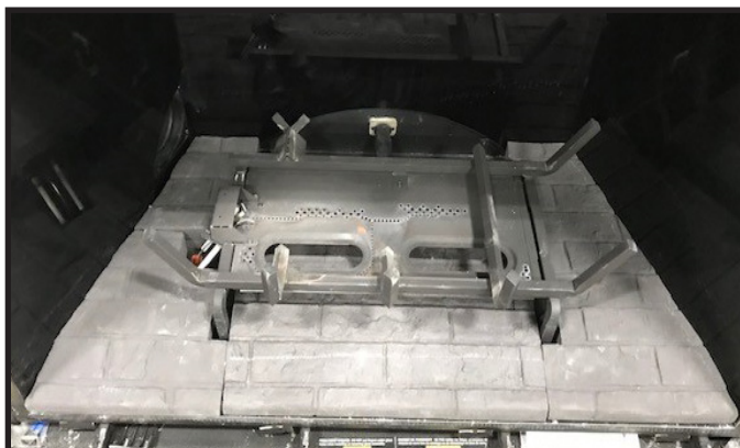
Figure 4 Lava Rock removed from appliance
