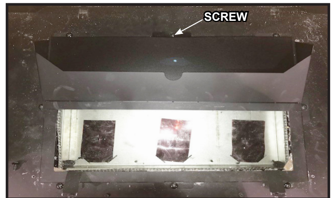
Figure 18 Reinstall Center Back Screw
