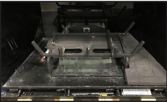
Figure 6 Left Base Refractory pieces removed from appliance
