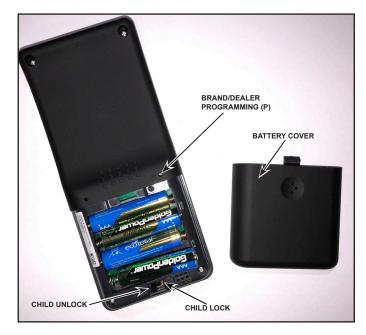
Figure 12 Install Batteries & Child Safety
