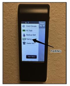
Figure 5 IFT2-RC450 Wall Mount / Pairing Screen
