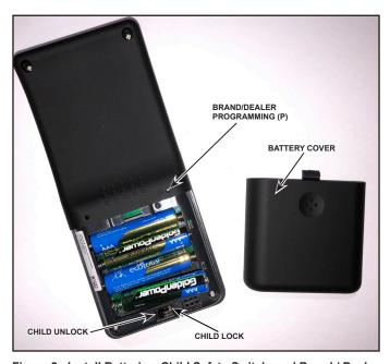
Figure 2 Install Batteries, Child Safety Switch, and Brand / Dealer Programming
