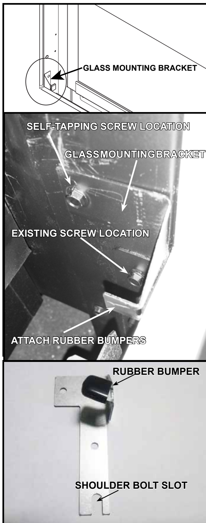
Figure 5.9 Install Glass Mounting Brackets
