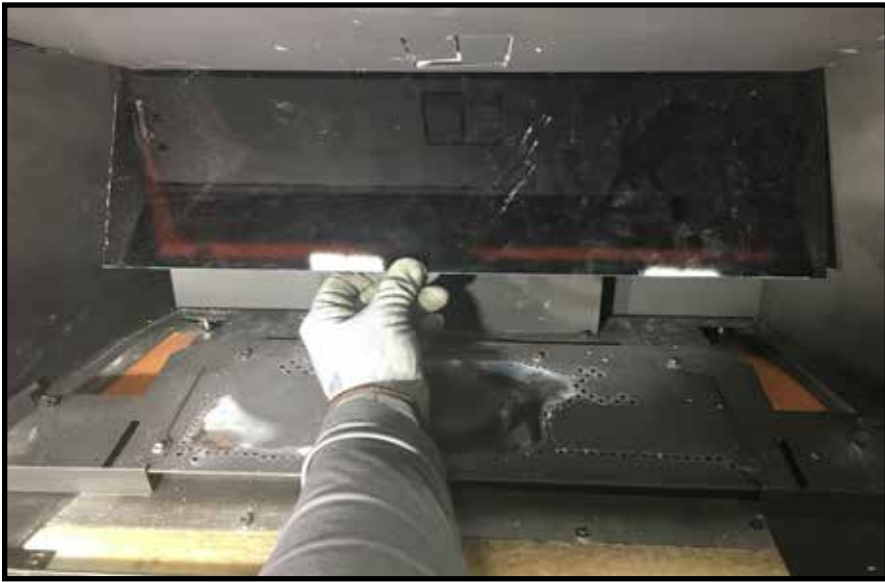
Figure 7 Install Rear Glass Panel
