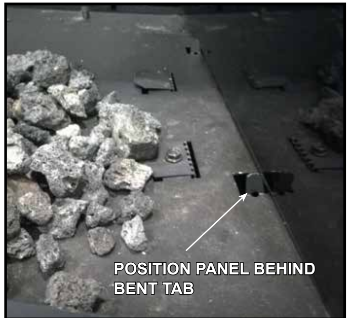
Figure 7. Side View of Bent Tabs
