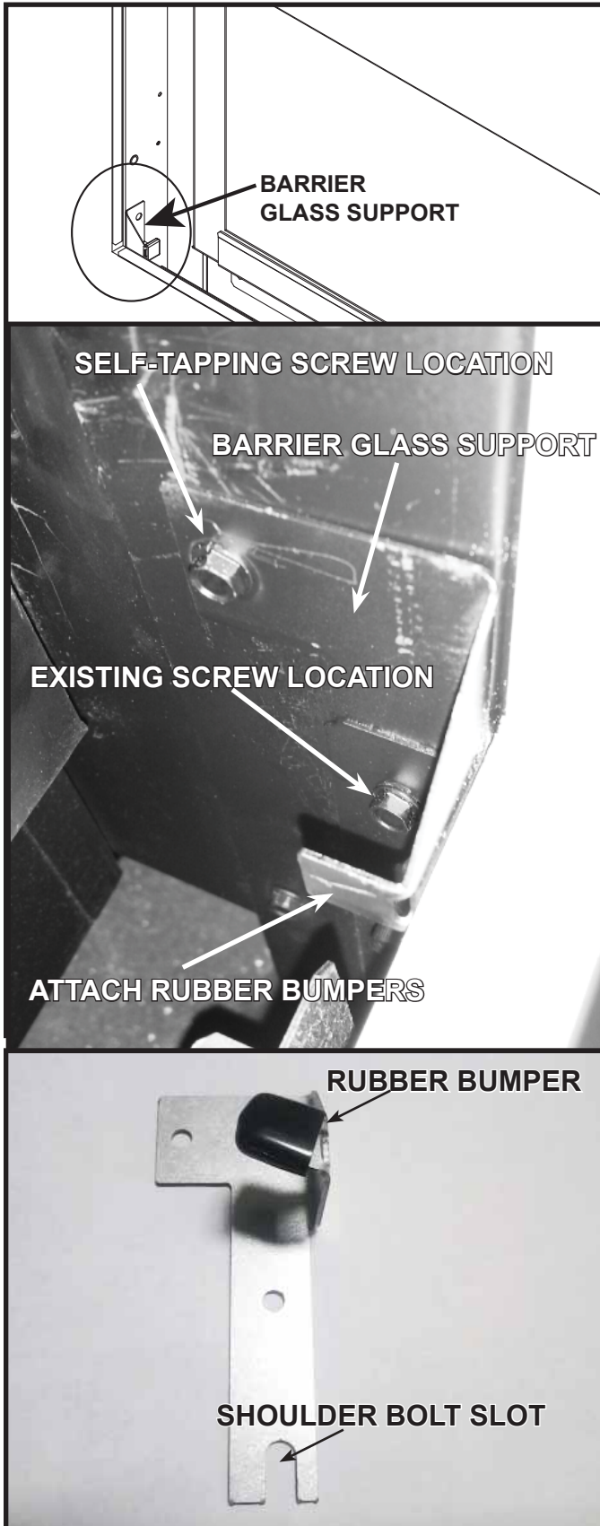
Figure 12. Install Barrier Glass Supports
