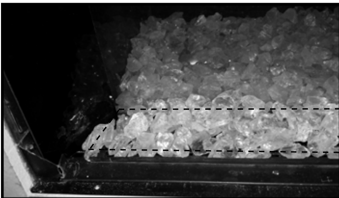
Figure 11. Place Media in Barrier Tray - PRIMO
