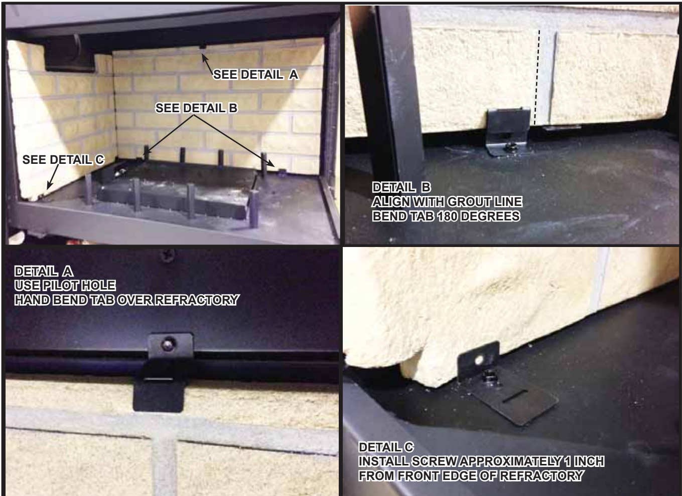
Figure 11. Fiber Back Refractory Installation Detail
