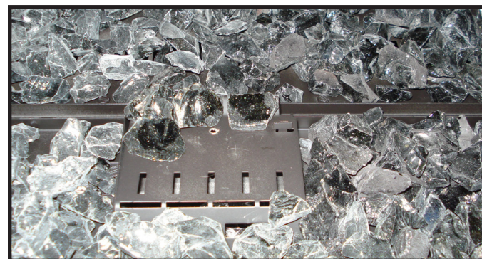
Figure 6. Place Flat Pieces of Glass Rock Media
