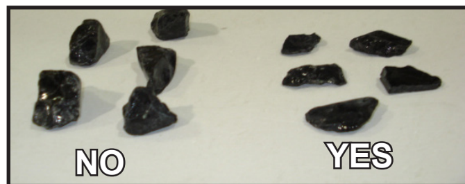
Figure 1. Selecting Flat Rocks for Pilot Cover.
