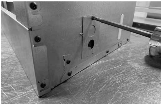
Figure 5.1 Junction Box Cover Removal
