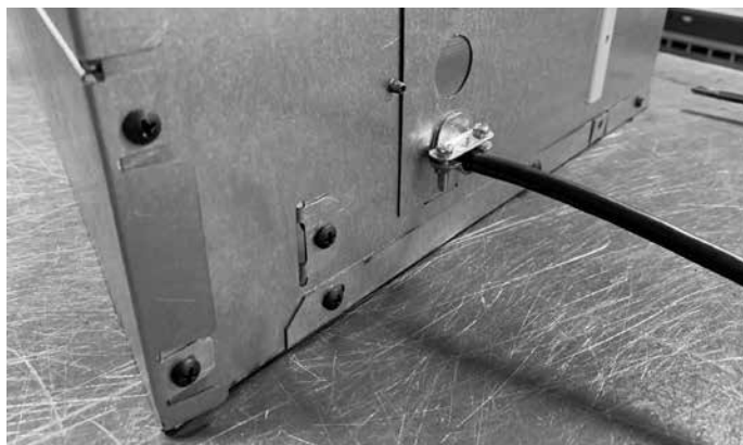
Figure 5.2 Reattaching Junction Box Cover
