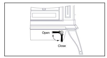
Figure 5.8- Turn the ashdoor handle clockwise to open and counterclockwise to close.
