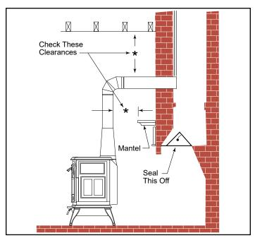
**Figure 2.6** - In this installation, the chimney connector attaches to the chimney above the fireplace opening.
