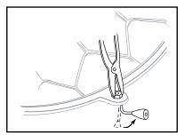
Figure 3.2 - Attach the griddle handle.
