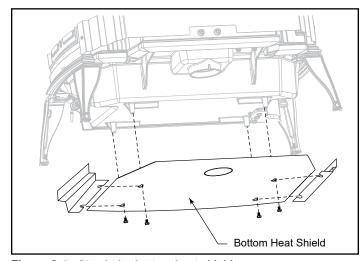
Figure 3.4 - Attach the bottom heat shield.
