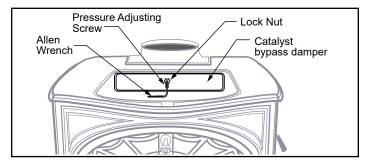
Figure 6.2 - Adjust the catalyst bypass damper with the Allen wrench.
