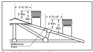
Figure 2.2 - The 2'-3'10' Chimney Rule.
