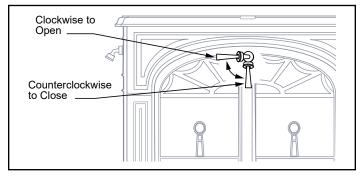
Figure 5.6 - To open the front doors, turn the handle clockwise.
