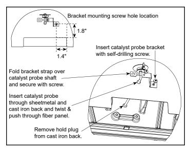
Figure 3.6 - Install the Catalyst Temperature Probe
