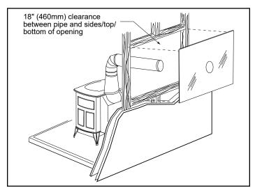
Figure 2.9 - An approved wall pass-through for Canada.
