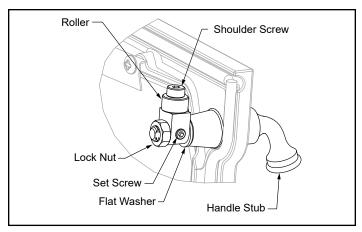
Figure 6.3 - Rotate pawl and/or remove flat washer to adjust latch.
