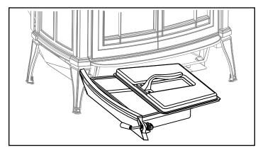
**Figure 5.9** - Be sure the cover is securely attached before removing the ash pan.
