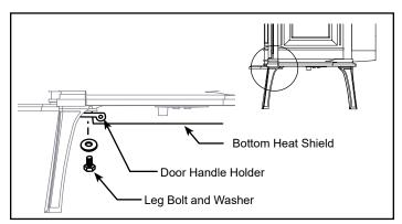
Figure 3.3 - Handle holder and heat shield positions.
