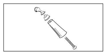
Figure 3.8 - Assemble the front door handle.
