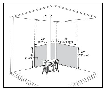
**Figure 2.14** - Parallel installation, vertical chimney connector, two wall shields. Reduced clearances for both rear and side walls. Wall shields may meet at corner if desired. Shielding for connector is centered behind connector.
