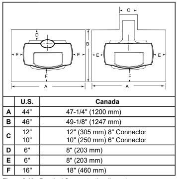
Figure 2.10 - Required floor protection dimensions.
