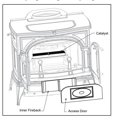
Figure 6.7 - Inspect the catalytic combustor.
