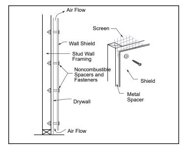
Figure 2.11 - Approved wall shield construction.
