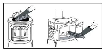
**Figure 5.5** - Top loading is the best way to add fuel during regular use. Front loading is useful for kindling a fire.
