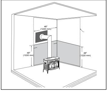
**Figure 2.15** - Parallel installation with rear wall pass-through, two wall shields. Reduced clearances to both rear and side walls. Wall shields may meet at corner if desired. Wall pass-through must comply with codes.
