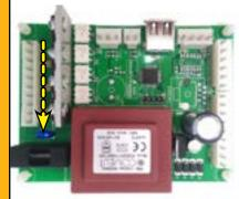
5. Remove the top of the black box to access the fuse. Check the fuse for any damage.
