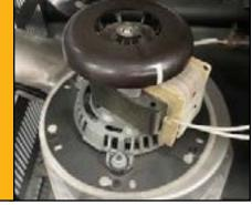
Loosen the 6 screws holding the blower motor onto the blower housing. You do not need to fully remove the screws. Twist the plate and remove the blower motor.
