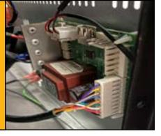
4. Locate the black rectangular box on the control board. Shown with the control board unplugged for better reference. Leave the control board in the stove.
