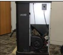
3. Remove the 2 screws holding the blower in place.
