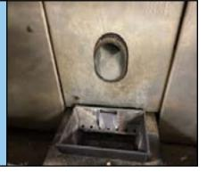
3. After cleaning the fire box area. Remove the fire pot and find the igniter chamber under the fire pot.
