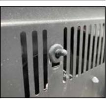
4. Locate the wire/ twist tie securing the ambient probe wire. Remove the tie so you can adjust the probe if needed.
