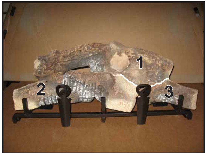
LOG NUMBER 3 (SRV768-705): Position log #3 onto grate such that tab D fits into slot on bottom surface of log. Push down until log is sitting flat on grate.
