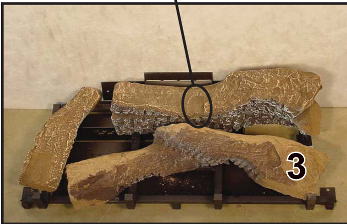
LOG #3 (SRV768-704): Position log #3 onto grate such that the tabs D and E fit into the slots on bottom surface of log and the right back side of log is flush against tab F.
