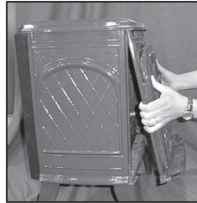
Figure 8.13 Lift up on the top of the Front, gently pulling out on the bottom. Set aside in a safe location.
