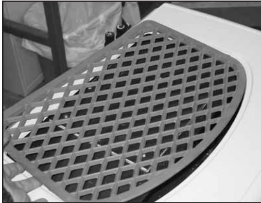
Figure 8.7 Place grille gently into the opening on top of the appliance.
