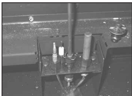
Figure 6.7 Use a 5/32 in. Allen wrench to remove the pilot injector.
