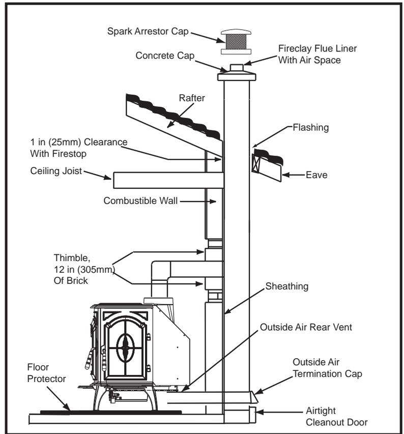
Figure 8.1 Masonry Chimney
