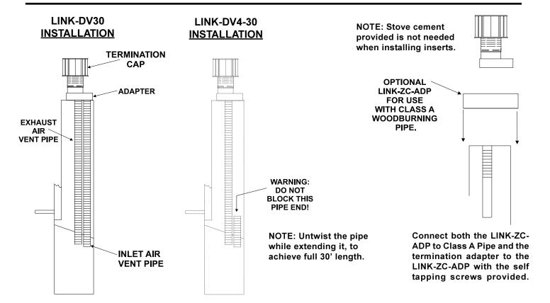
**WARNING:** The exhaust pipe must only be connected to the exhaust starting collar of the unit and the center of the termination cap.
