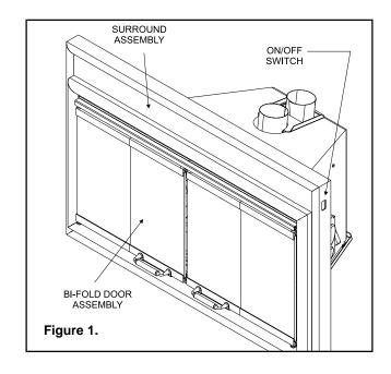
pilot for the masonry screws (blue). Re-attach outer surround assembly by completing Step 2, then anchor the outer surround with the 3/4" self drilling sheet-metal screw at center by driving screw into pilot hole in anchor bracket (see Figure 2). The decorative surround will pull tight against fireplace front.
