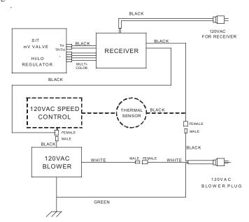
Connect the 30" long 18AWG wires labled "120VAC FAN ONLY" between receiver and blower as shown in the follwing diagram as well.
