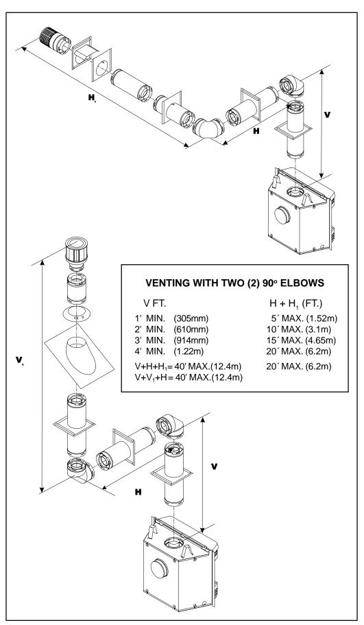
Figure 12. Venting with Two 90° Elbows
