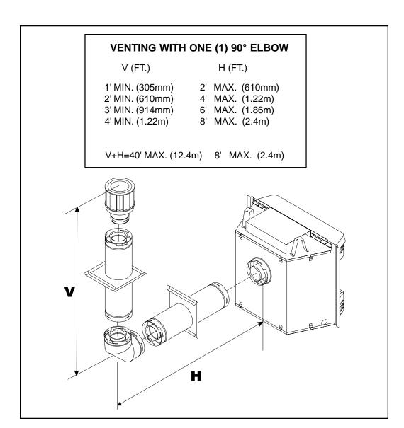
Figure 8. Venting with One 90° Elbow
