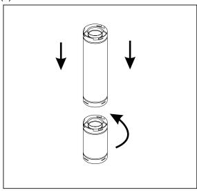
**Figure 17. Adding Venting Components**
