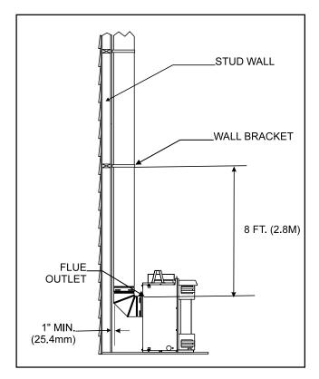
Figure 18. Installing Support Brackets
