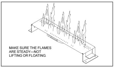
Figure 36. Burner Flame Patterns
