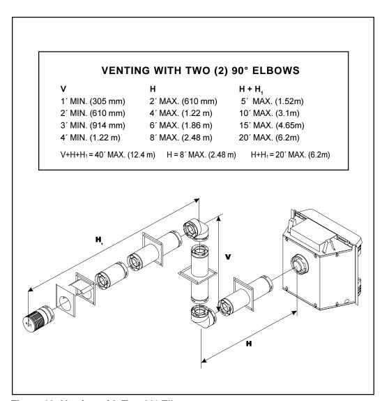
Figure 10. Venting with Two 90° Elbows
