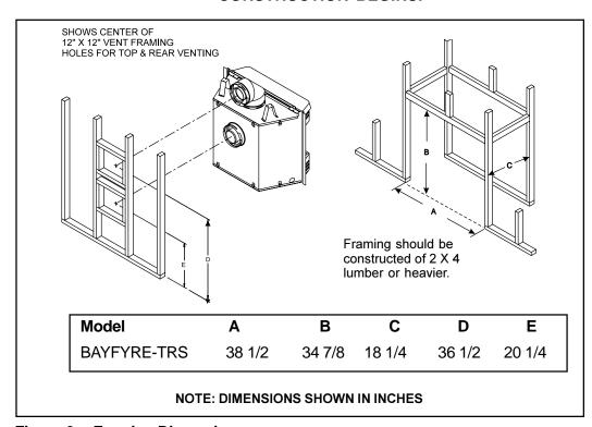
Figure 3. Framing Dimensions
