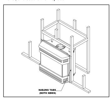
Figure 27. Proper Positioning, Leveling, and Securing of a Fireplace
