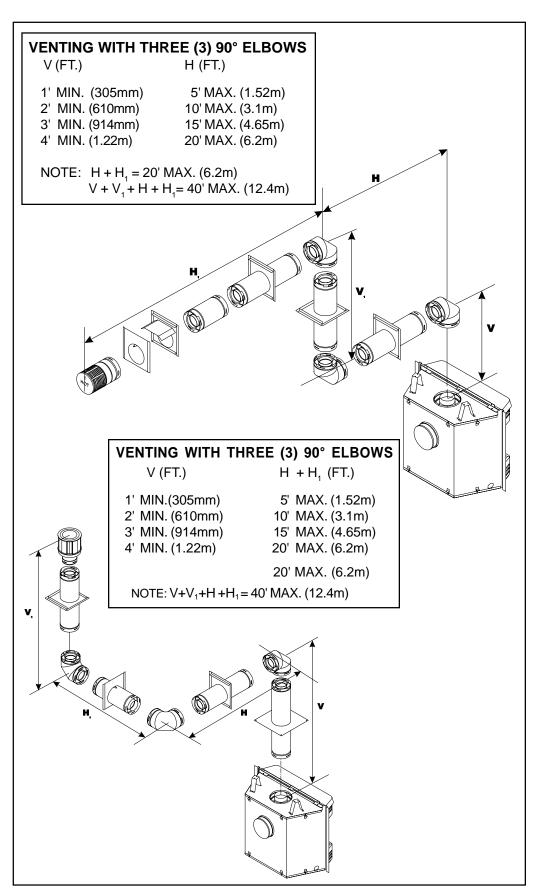
Figure 14. Venting with three 90° elbows
