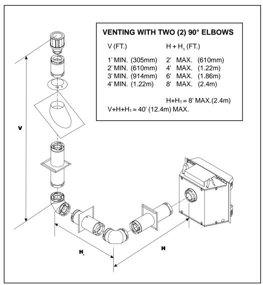
Figure 11. Venting with Two 90° Elbows
