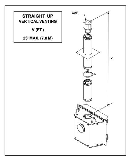
Figure 6. Straight Up Vertical Venting
