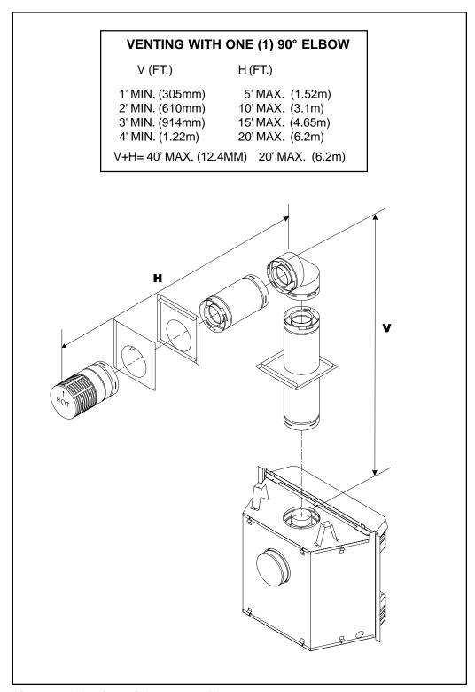
Figure 9. Venting with One 90° Elbow
