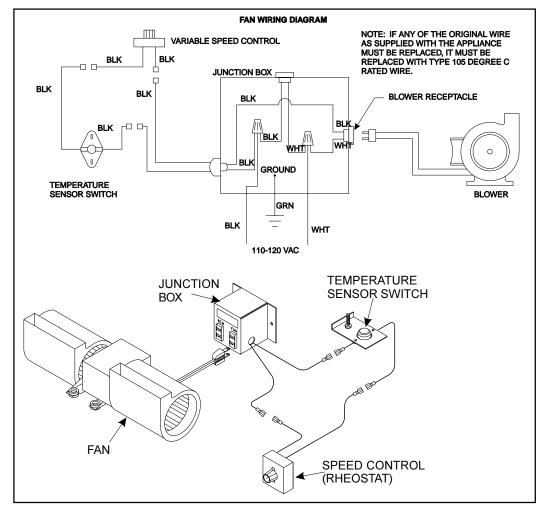
Figure 31. Fan Wiring Diagram
