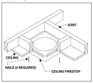
Figure 22. Ceiling Firestop (Ceiling Side)
