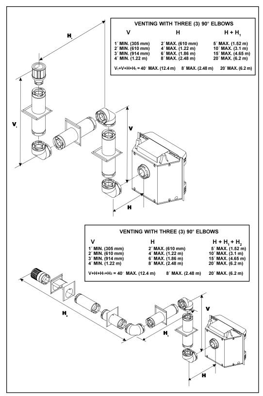
Figure 13. Venting with three 90° elbows
