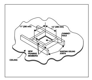
Figure 21. 11" x 11" Hole and New Framing Members
