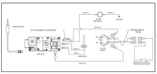
Figure 30. Standing Pilot Ignition Wiring Diagram
