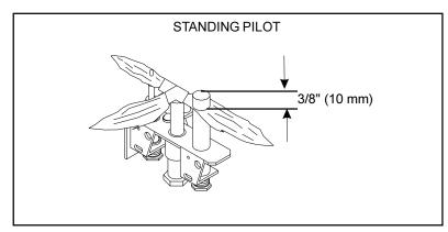
Figure 37. Pilot/Ignitor Flame Patterns
