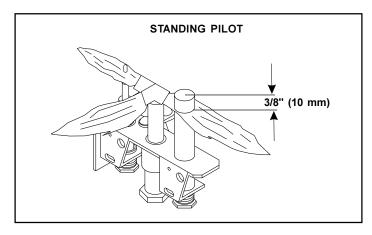
Figure 28. Gas Controls Systems
