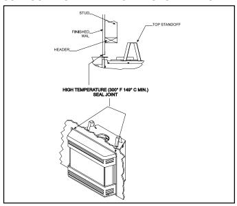
Figure 33. Sealant Material
