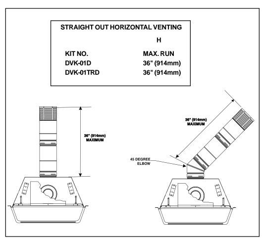
Figure 7. Straight Out Horizontal Venting
