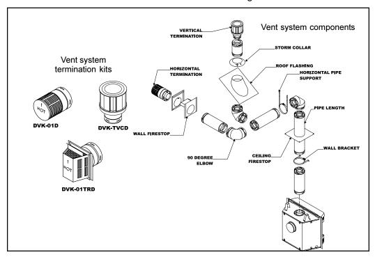
Figure 4. Vent Components and Terminations
