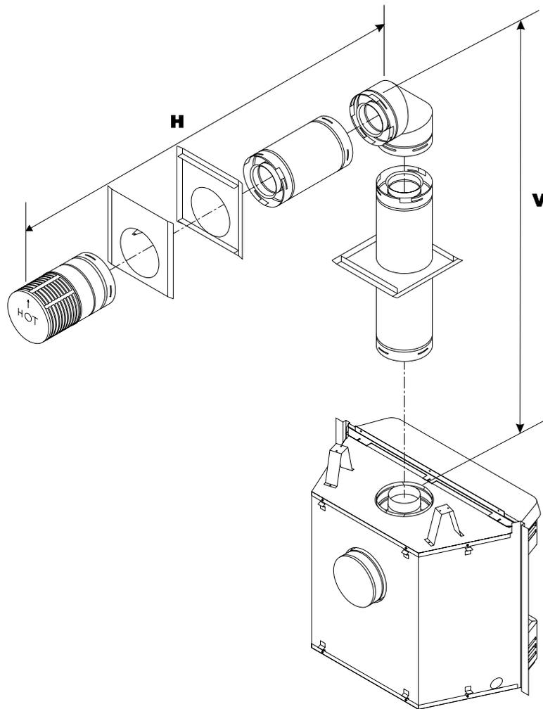
**Figure 9. Venting with One 90° Elbow**
