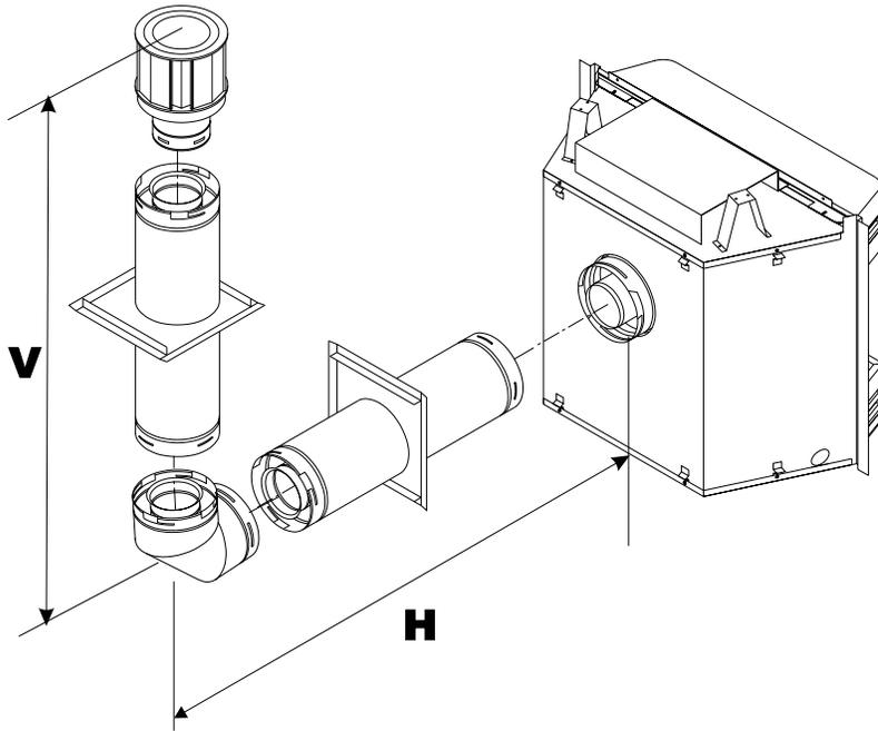
Figure 8. Venting with One 90° Elbow
