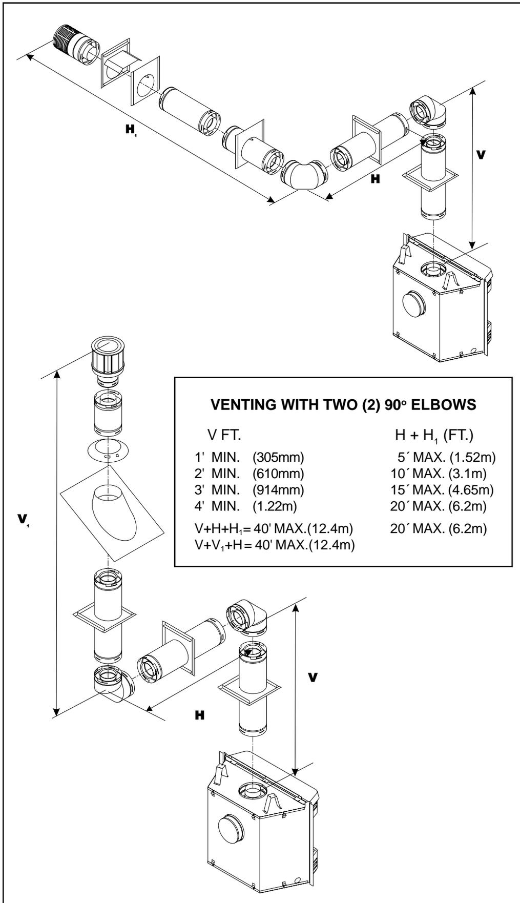
Figure 12. Venting with Two 90° Elbows
