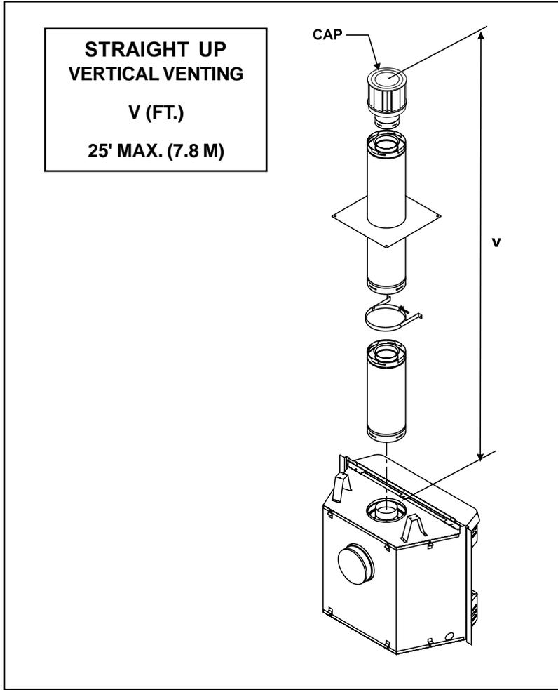
**Figure 6. Straight Up Vertical Venting**
