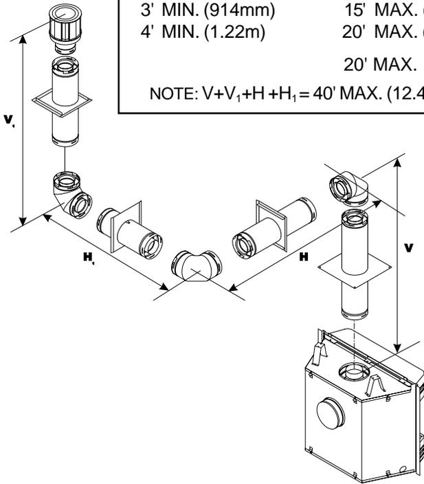
Figure 14. Venting with three 90° elbows
