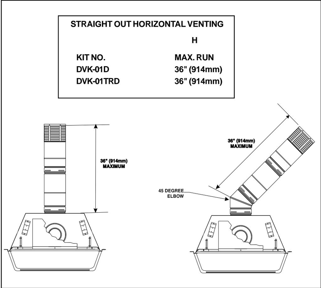
**Figure 7. Straight Out Horizontal Venting**
