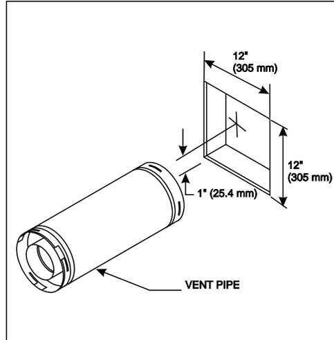
**Figure 19. 12" x 12" Hole and Vent Pipe**
