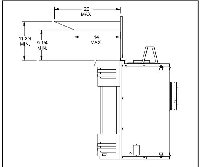
**Figure 32. Minimum Vertical and Maximum Horizontal Dimensions of Combustibles above Fireplace**
