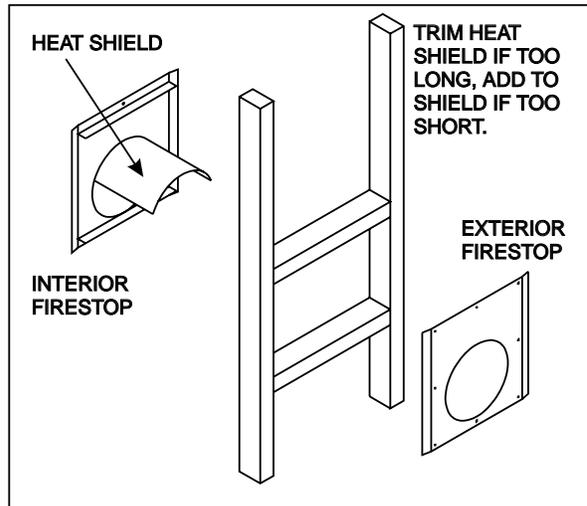
**Figure 20. Heat Shield, Interior and Exterior Firestops**
