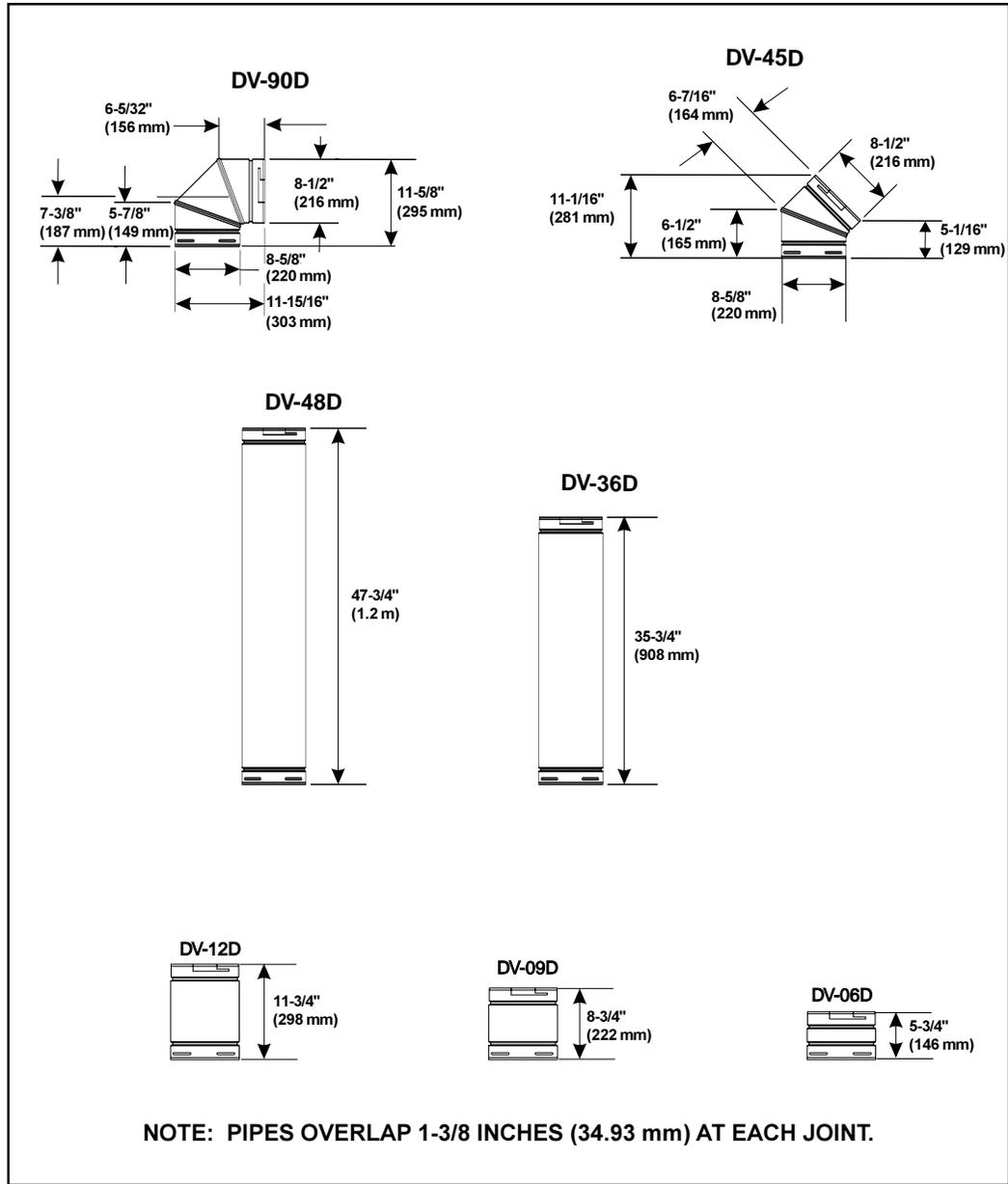
**Figure 5. D-Series Direct Vent Component Specifications**
