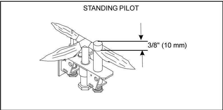
**Figure 37. Pilot/Ignitor Flame Patterns**
