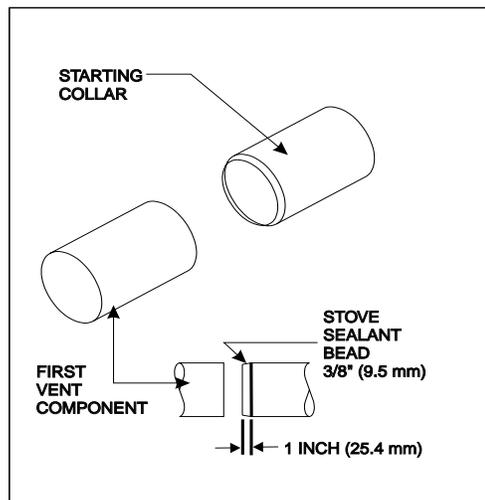
Figure 16. Attaching the First Vent Component to the Starting Collars
