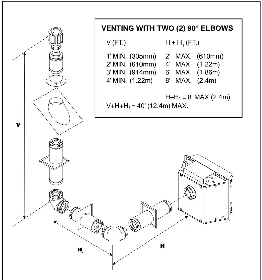
Figure 11. Venting with Two 90° Elbows
