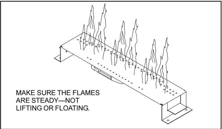
**Figure 36. Burner Flame Patterns**
