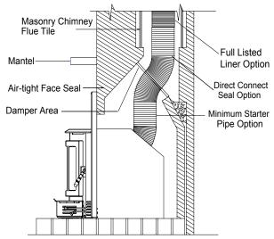
Figure 9A - Installation Into Masonry Fireplace
