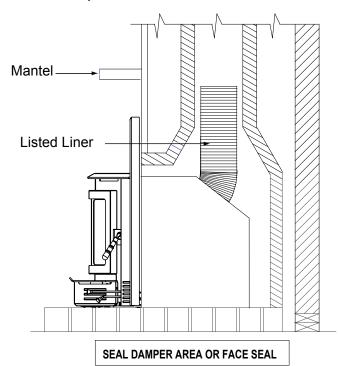
Figure 10A - Installation Into A Factory-Built Zero Clearance Fireplace
