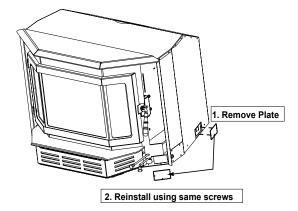
Figure 8A - Installing Outside Air
