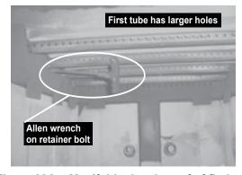
Figure 20A - Manifold tubes in roof of firebox.
