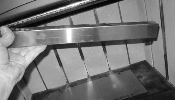
Figure 4.5 Removing Baffle Protection Channel
