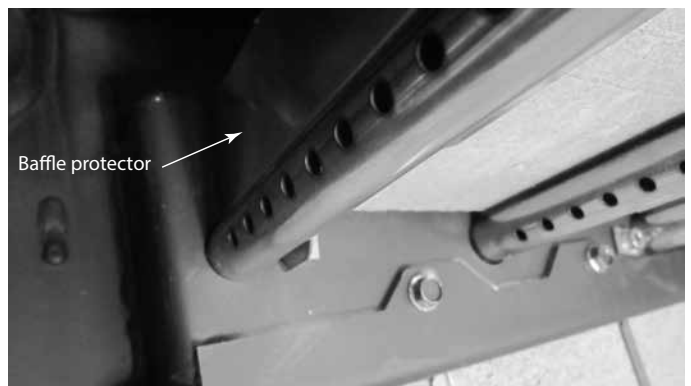
Figure 4.9 Reinstall Baffle Protection Channel
