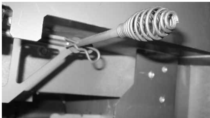
Figure 4.36 Reinstalling Hairpin Clip and Washer
