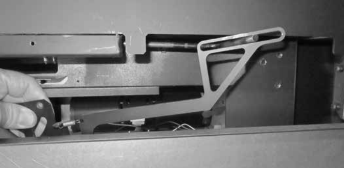
Figure 4.23 Inserting Timer Assembly
