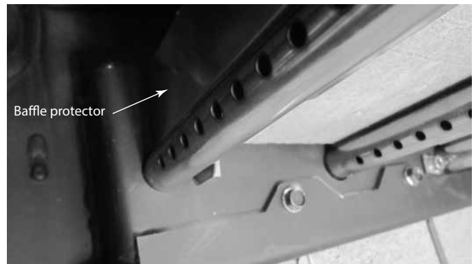
Figure 4.9 Reinstall Baffle Protection Channel
