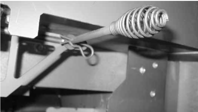
Figure 4.25 Reinstalling Hairpin Clip and Washer
