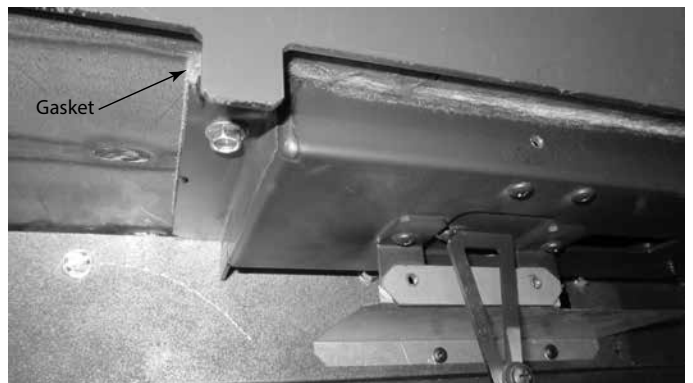
Figure 4.22 Install New Air Chamber
