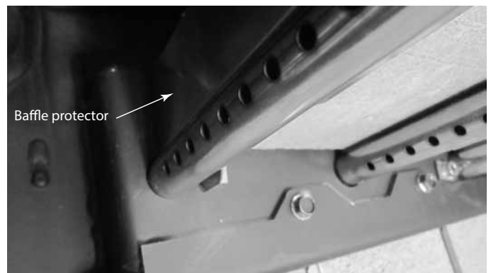
Figure 4.9 Reinstall Baffle Protection Channel
