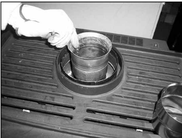
Figure 10 Remove SL-D Adapter
