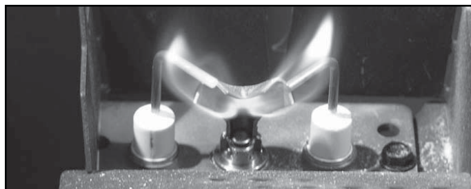
Figure 3.1 IPI Pilot Flame Patterns
