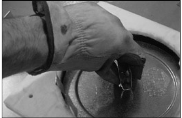
Figure 7.4 Remove Vent Cap
