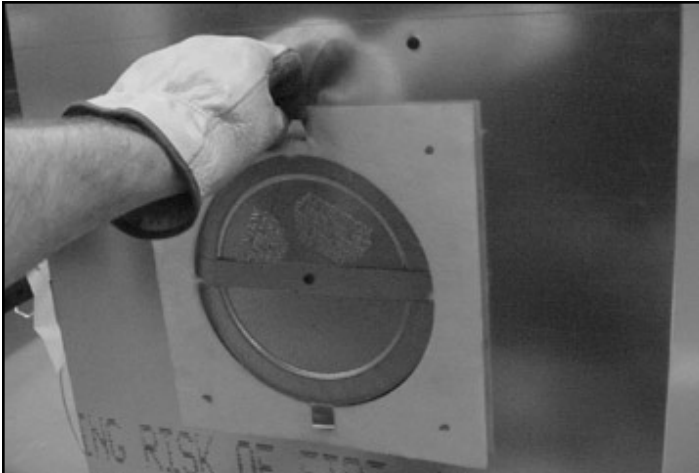
Figure 7.7 Remove Insulation Gasket
